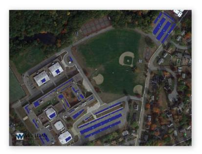
Figure 28. FS Solar PV Layout (52.8 kW)
