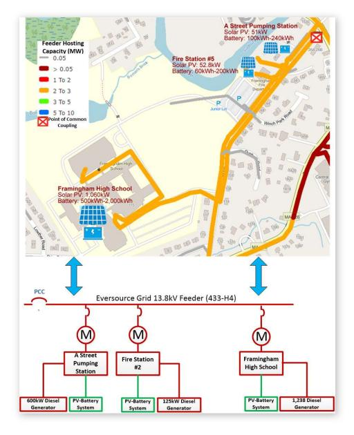
As shown in **Figure 1**, all the stakeholder locations are fed by the 13.8kV feeder. This configuration served to reduce the complexity of community microgrid islanding and interconnection.
