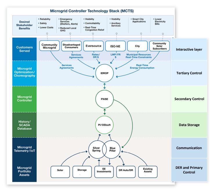
In microgrids, the primary control offers a localized control in real-time, designed to realize load sharing among parallel-connected DERs without needing communication channels between DERs.
